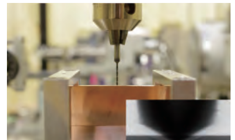
③ ドリル加工の高速X線撮像 High-speed X-ray imaging of drilling
