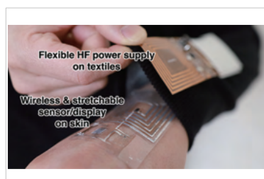
3 Wireless soft sensor and display system
