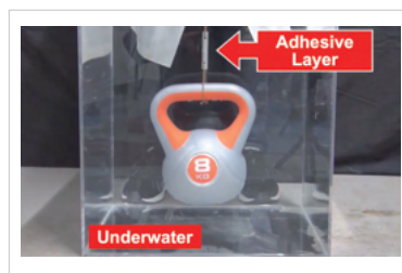
1 The two aluminum rods were joined together underwater and lifted a weight.
