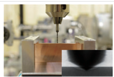
3 High-speed X-ray imaging of drilling
